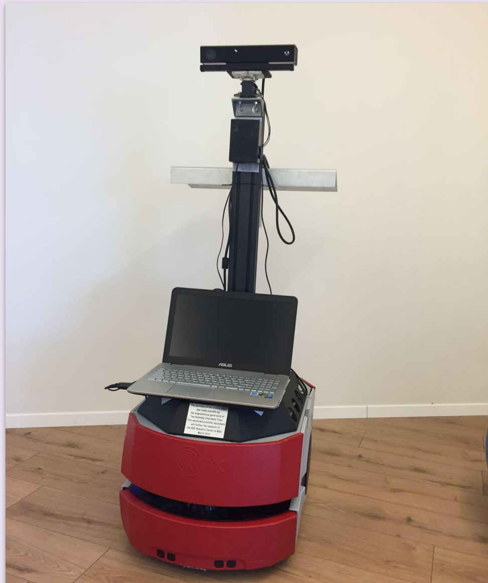
Figure 1. Experimental robot setup based on the Pioneer LX Robot
