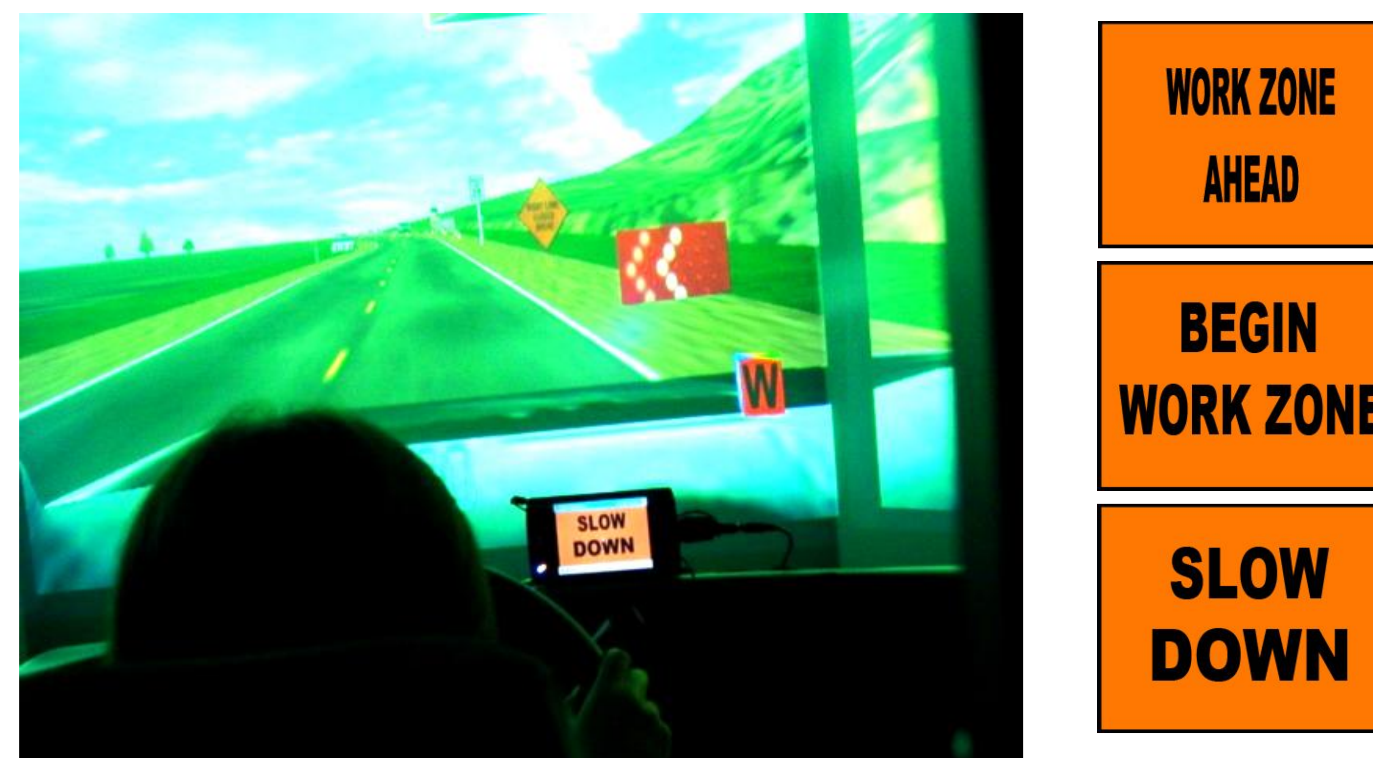
Fig. 1 Left: Experimental setup in the visual condition (visual warning are presented to the right of the driver) Right: Images of the visual in-vehicle warning messages.
