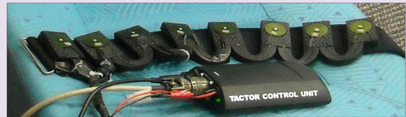
Figure 2. The Vibrotactor belt and the Eval2.0 controller.
