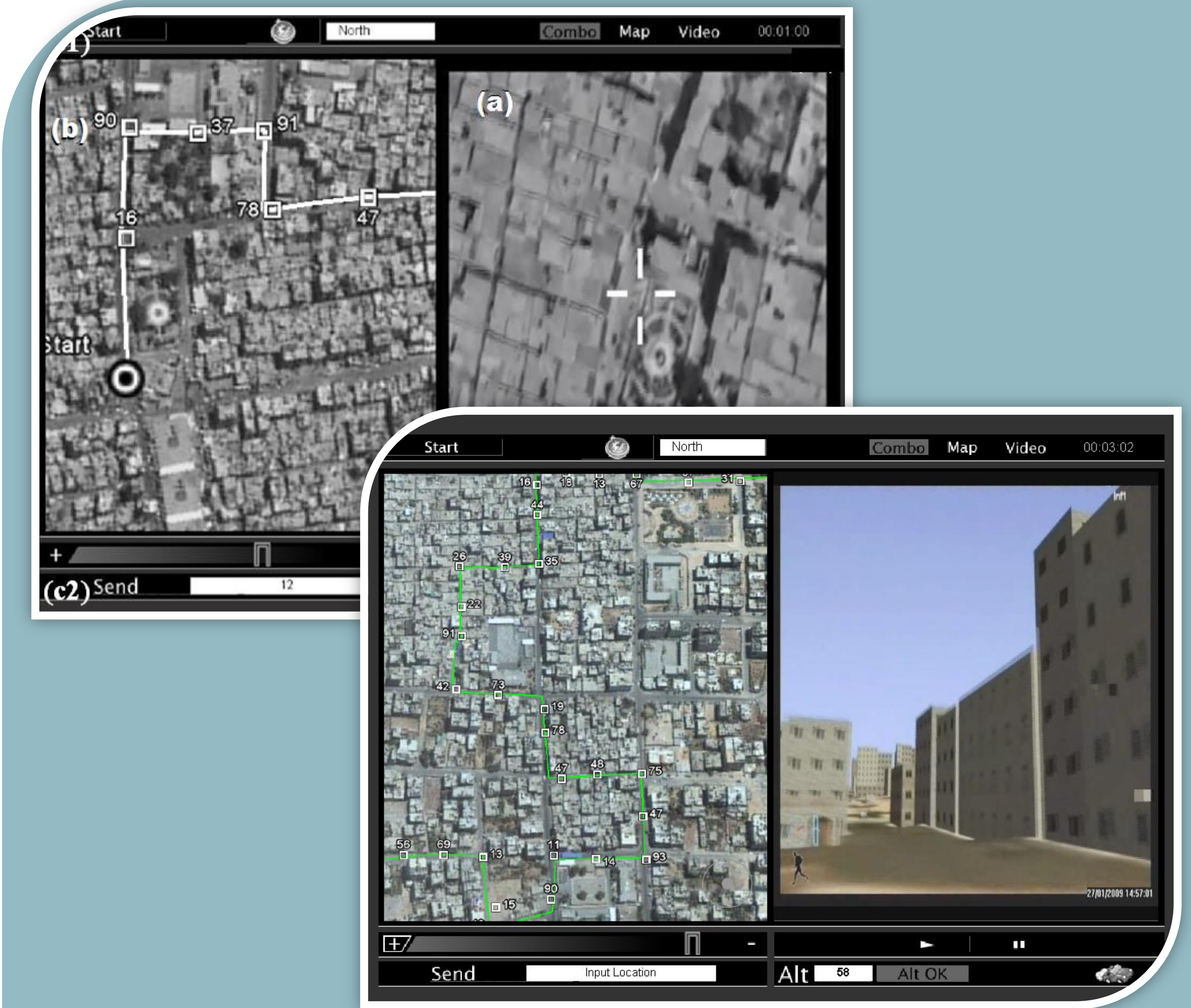
The experimental system interface. (Right) video feed. (Left) topographic image of the area, from a (top) UAV B/W perspective Vs. UGV colored one
